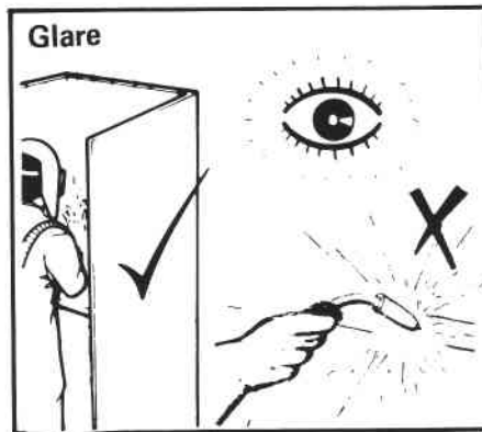
Wear your headshield (or face screen) and screen the welding area.
