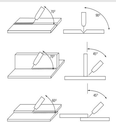
For fillet and lap welds superior weld appearance is achieved using a torch angle of 60/70°, and a forehand technique (pushing). This results in a more even distribution of weld metal, accompanied by a slight reduction in penetration.
