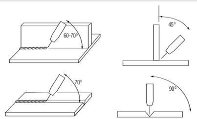
In certain circumstances the forehand technique i.e. pushing, can be used to advantage. On small fillet welds where penetration is not of paramount importance the higher welding speeds required are such that the molten slag is prevented from running ahead of the weld pool. This also has the advantage of producing a mitre fillet where as the backhand method tends to produce a more convex profile.
